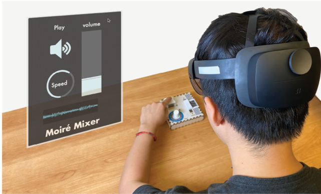
Figure 8: We integrate multiple widgets to create an audio console that controls a music interface that can be used for AR.
